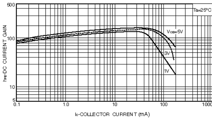
Fig.3 DC current gain vs. collector current (I)
